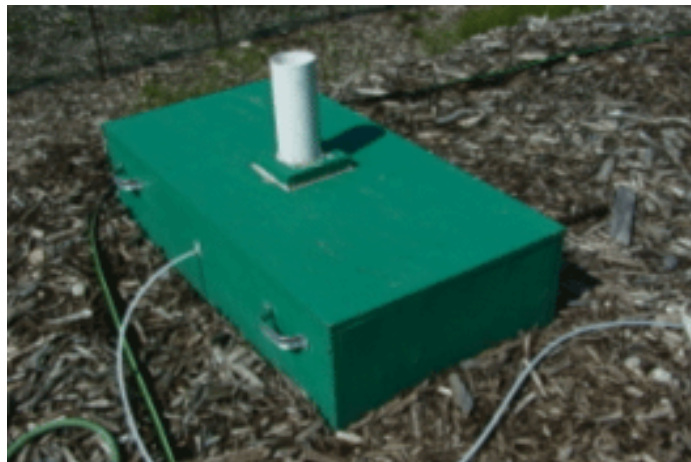
FIGURE 4 - BIOFILTER FUME COLLECTION HOOD
